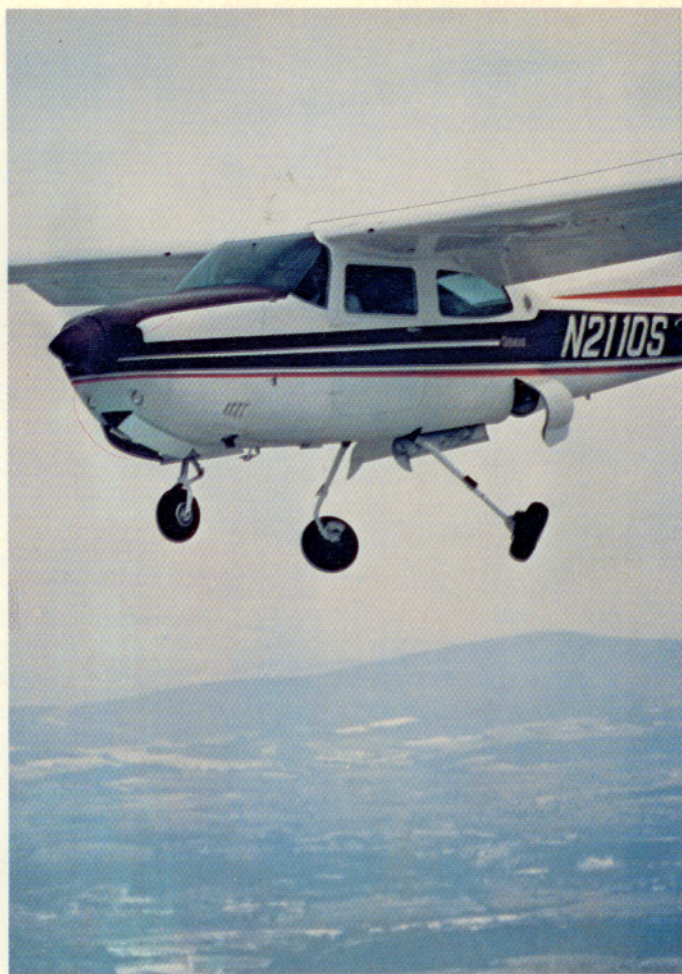
Main gear rotates during cycling process, and gear doors stay closed at all other times.
