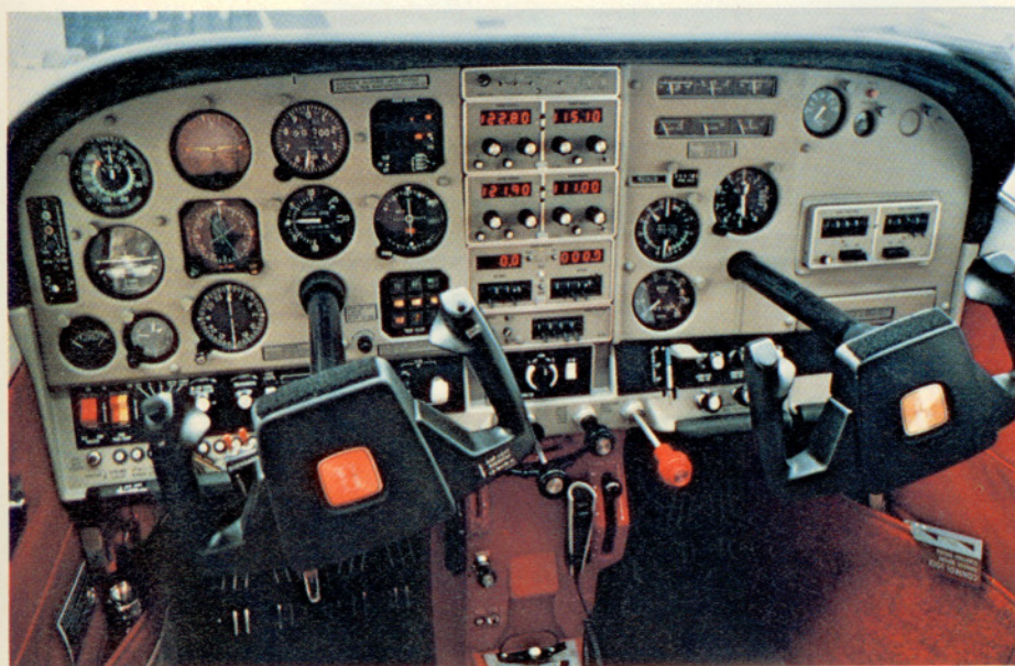
Installed on the craft were an integrated flight director and autopilot, DME and RNAV. Heavily padded yokes blocked vision of parts of the panel.
